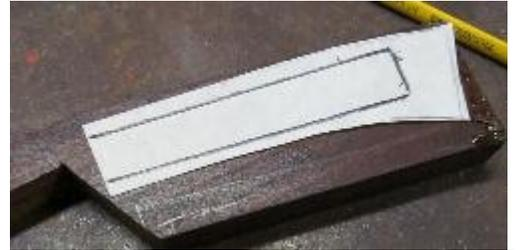
The idea is to split the block taking into account the offset due to the tang thickness (here 0.105"). Given a block of 0.758", the midpoint would be 0.379". Move that 0.105/2" to one side and the thickness of the two scales is known.
