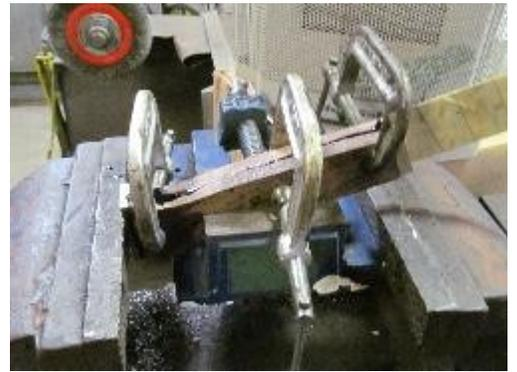
The next step is to insert the 1/8" pins and jazz the handle up with mosaic pins. The tooling needed is shown here = a drill the size of the mosaic pin to be used (#2 at 0.221" – and I don't remember where I got 5.6mm tubing to make the pins), a depth indicator, a saw jig and the Allen wrench needed for the jig.
