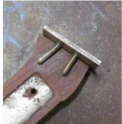
But for this blade, I elected to make a “T” block which fits into a milled recess and is riveted into place. Following the same procedure as outlined above for the tang...
