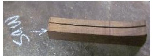
If the outer surfaces are clean and flat, all you have to do is flip-flop the blocks left to right and the smooth surfaces are now inside and the saw marks are outside.
