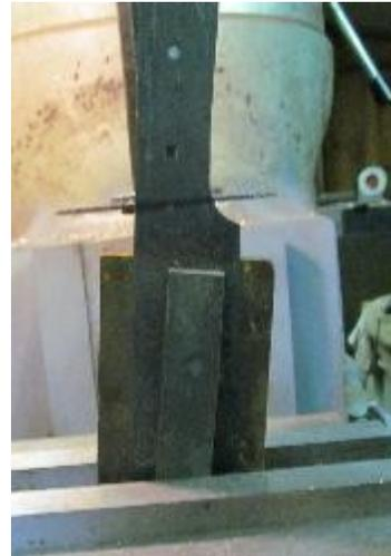
The blade was positioned at a slight angle (because I think it just looks cooler!) and the saw was moved to the left and positioned with the axis of rotation of the saw perpendicular to the tang's dorsal surface (ok – the spine...whatever). The mill was SLOWLY cranked to the left and to create an approximately 3/16" slot.
