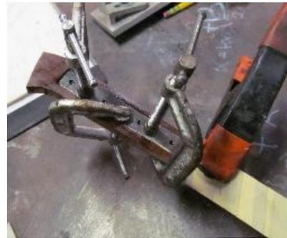
The 1/8” pin holes were drilled and the other scale fitted. When the fit of the guard to the scale was acceptable, the scale was clamped to the blade and the holes drilled through the second scale. Alignment pins will be used when the second scale is to be glued in place. Note that the second scale is also oversized.
