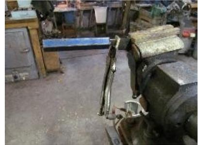
I use TIX solder and the MAPP gas torch shown here does the trick. Note the torch holder on the tank. I start from the tang side and will eventually have to flip the blade over. The holder means I don't have to turn off the torch or have it go wandering during the flip operation.
