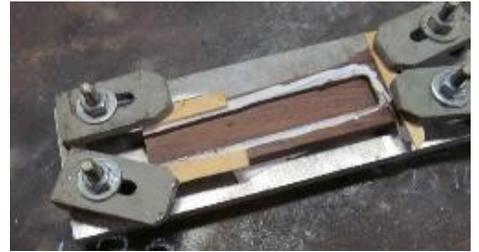
The tang fits with no difference in wood-to-metal detected by running a finger tip over the interface at the guard. It literally snapped into the recess. The scale was deliberately oversized and the wood to be removed is delineated with a white pencil.
