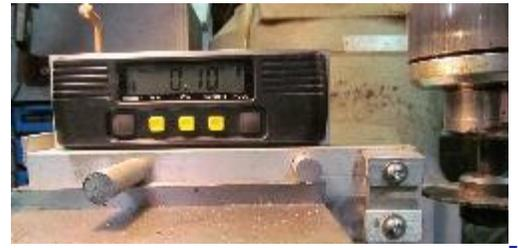
The removable peg is pulled and the jig is rotated downwards until the protractor reads the correct angle. Given the 5/16x18 bolt (peeping over the left of the protractor), there are 0.055" per rotation. The distance between the pivot point and the bolt center is 5.2", Using the same equation,  $\arctan[0.055/5.2]$  gives 0.6° per revolution, so a little over two turns ought to be close (for those without a cool digital protractor)
