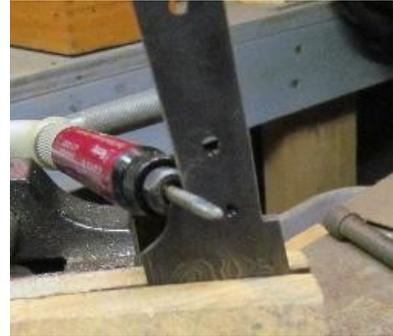
The image to right shows the radii and the offset of the slots. The 3/32” hole in the midline of tang was intended for a rivet holding two bolster blocks to the blade. Guess what isn't really needed. Oh well...
