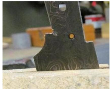
The next step is to cut a “V” slot in a block of guard material. Using a dial caliper, the dimensions are shown at the right (units are in 1/1000”). There is about 0.025” difference between top to bottom over a 0.768” run. A bit of trig indicates that a 1.3° angle is needed relative to the dead center of the tang.
