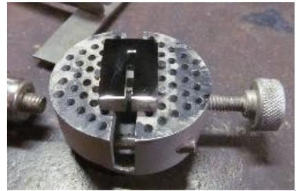
The next step is to make sure the fit is within soldering limits. A vise grip is used to “close” the ‘U’ and a piece of square tubing is used to tap the guard solidly onto the shoulder.
