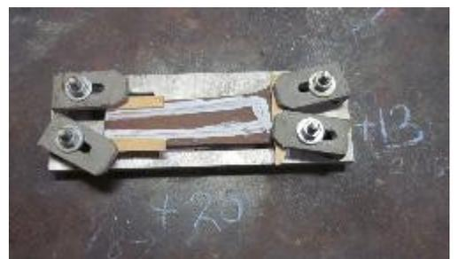
The next step is to fire up the mill – here with a 3/16” 2-flute end mill and running at high speed. Just trace out the recess and keep blowing off the chips to see what to cut next. Etch-a-Sketching is a very accurate description.
