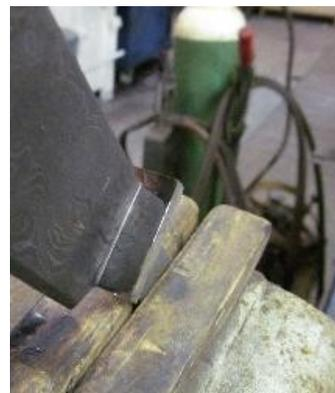
Here is the other side. Note that the guard is close to correct at the ventral side of the tang and I have a bit of nickel silver to remove at the dorsal side.
