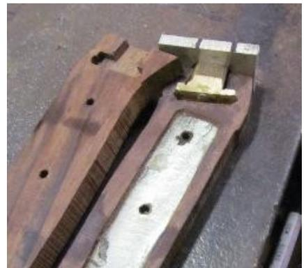
The solution is shown here. Use a small drill press vise (2.5") to hold the pommel perpendicular to the vise's jaws. The whole assembly is then placed in a machinist vise and the pommel is pressed to the mating surface. Once the epoxy sets up inside the pommel recesses, there is no way anything can come loose without destroying the handle first.
