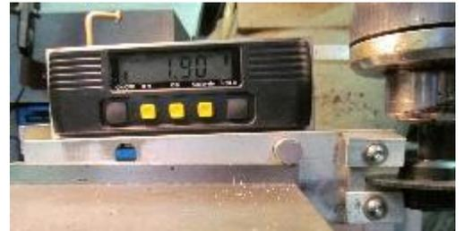
The table is cranked to the right by the depth of the slot (in this case, 0.767"). The saw is withdrawn and the jig is cranked up to the same angle on the other side of dead level. The table is then adjusted so the cut will form the other side of the slot taking into consideration the 0.080" thickness of the saw. Depending on whether the slot widens or narrows to the left, you'll have to do some thinking.
